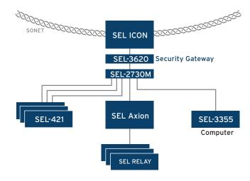
In this example of a substation network, the SEL-2730M supports engineering access, SCADA, synchrophasors, and many other required services with easy-to-use configuration.
